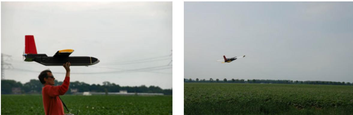
Figure 38. Operator launching an unmanned aircraft over a potato field via a launch rope. The plane then flies autonomously following a pre-programmed flight path.
