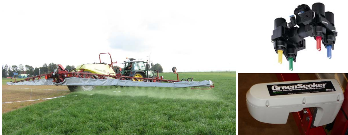
Fig. 1. VarioSelect nozzle holder and GreenSeeker sensor placed on the spray boom, sprayer sprays a high volume above green grass (right) and a low volume above desiccated grass (left).
